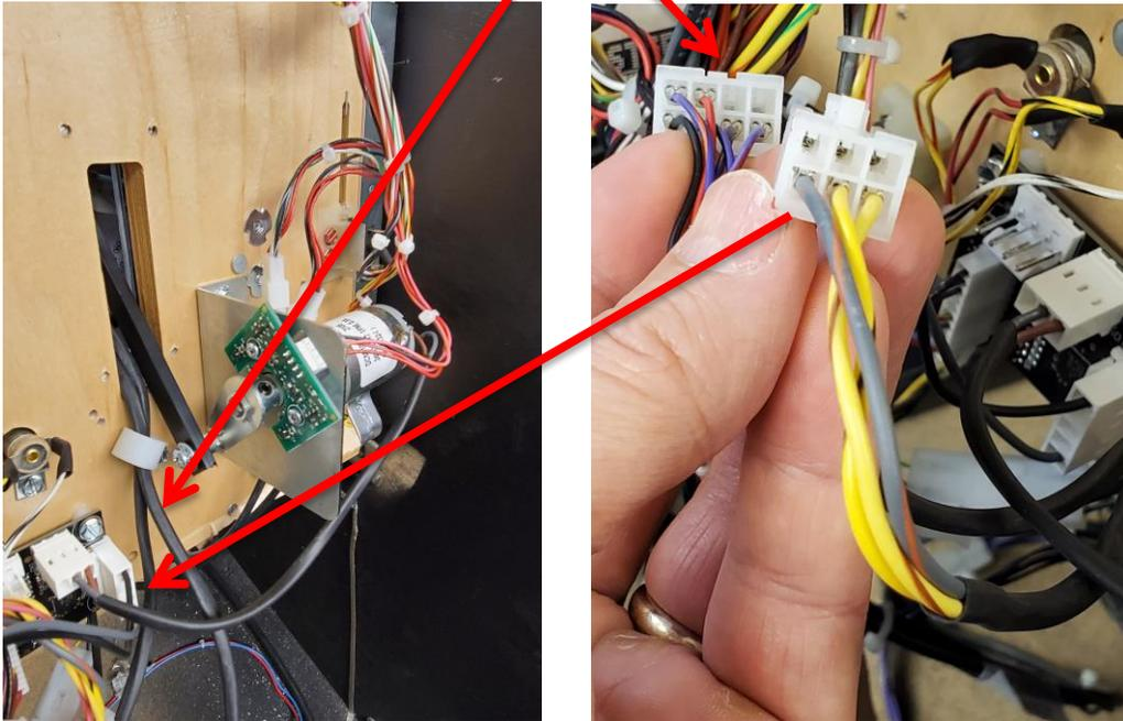
**Once all the hardware has been removed and the Mini playfield harnesses are disconnected, carefully raise the mini playfield away from the pivot brackets. This should give you access to the mini playfield harness and allow more room to disconnect the harness from the mini playfield.**
