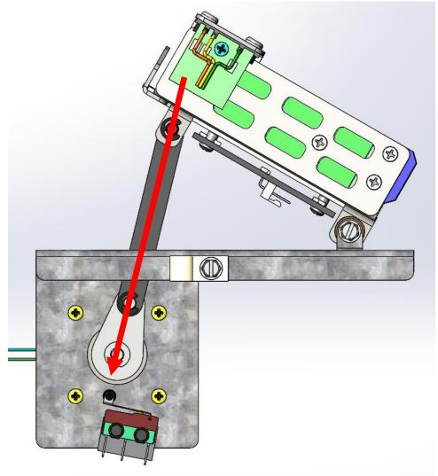
time machine ramp is probably not aligned properly in the up position. When in the up position the ramp link (black piece), and the lifter needs to be inline. This can be adjusted in the Ramp adjustment's menu, and the up position value can be adjusted. Move the value up or down until the link is inline with the lifter. This should make the ramp mechanically locked in the up position and the ramp won't move.
