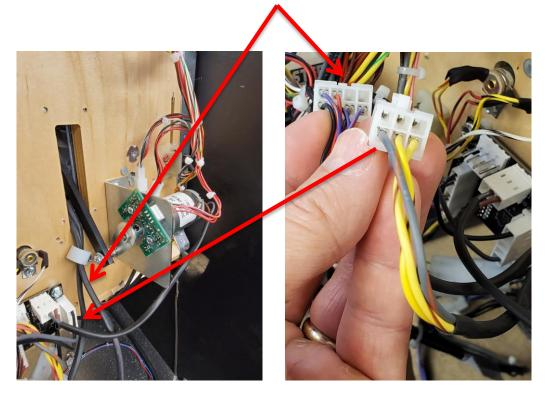
Once all the hardware has been removed and the Mini playfield harnesses are disconnected, carefully raise the mini playfield away from the pivot brackets. This should give you access to the mini playfield harness and allow more room to disconnect the harness from the mini playfield.
